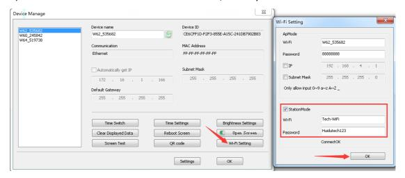
4). The PC connected the Wi-Fi signal, and open HD2016 Software, it can find All the Wi-Fi cards.
