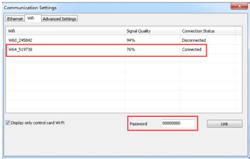
3)After connected the WIFI, in software it can find the device.
