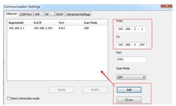
2).wifi: Used connect wifi signal of controller ,automatically default input password 88888888 ,no need manual input, as below shows:
