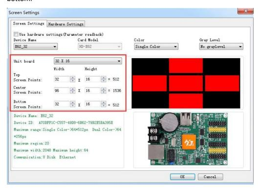
2). Cross sign screen can establish Global program and normal program, global program separated the top widdle and bottom and showing in one area. Establishing program can set up 3 areas to show program.
