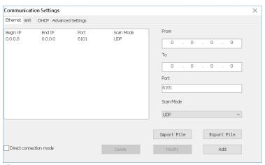
②.when not select "Direct connection mode", it is suitable for condition when controller and main operated PC are not at the same network segment, it need add the IP address of controller network segment to the software. Operation as below. After added, then you can find the controller in 192.168.3.\*
