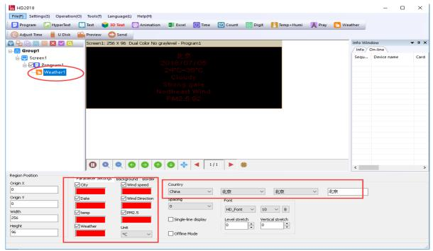
1. The controller will obtain the weather data every hour (directly from the server);
